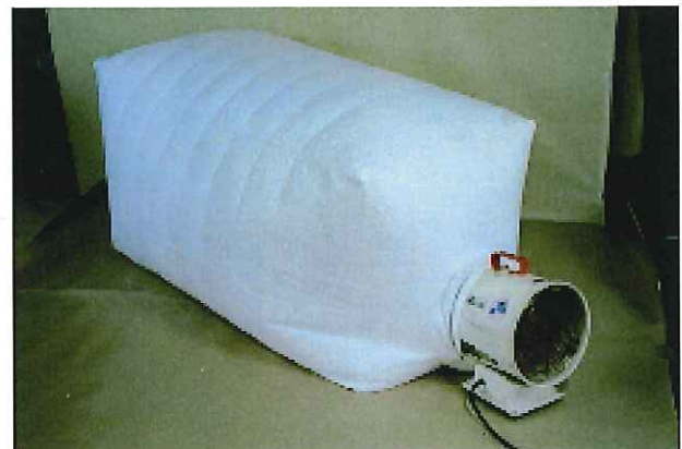
Simplified dust removal filter, which can be used by simply attaching it to a fan
