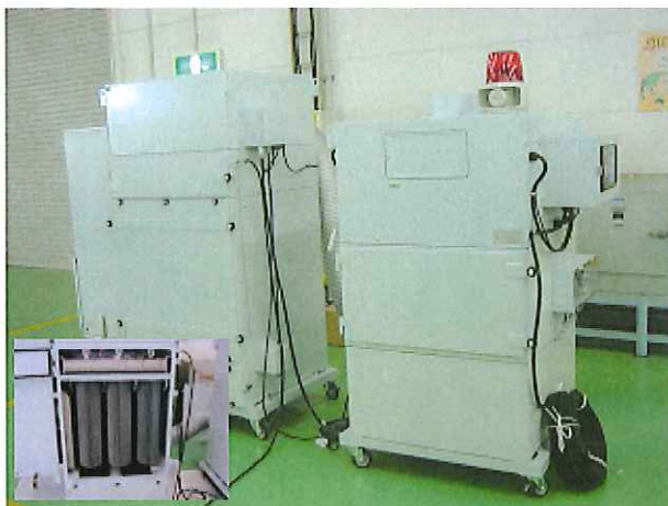
JER-FC, Fume collector equipped with automatic brush-off mechanism
